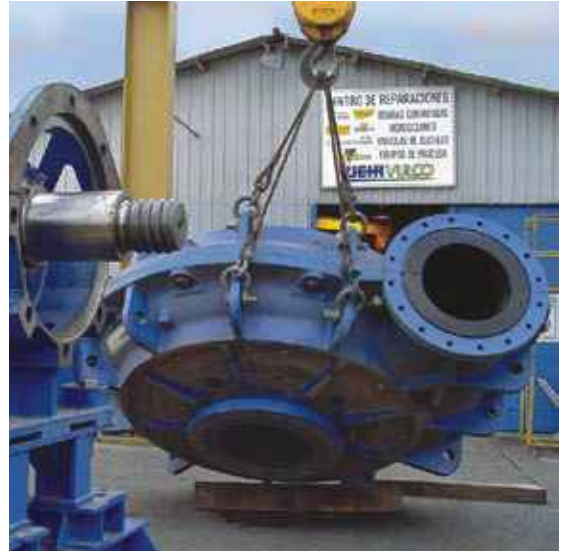
Above: A new innovative quick change procedure has been developed for faster removal of the larger MC range pump wet ends. A 650 MCR wet end being removed in Santiago, Chile
