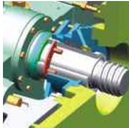
Left: Orange centering tool pins align stuffing box to the sleeve
